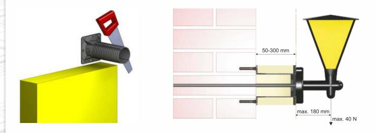
There is necessary to cut the carrier including inserted insulation before installation depending on layer thickness insulation.
